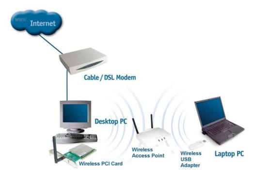
Please note that this type of installation requires that your ISP (Internet Service Provider) provides you a static IP address for each computer and the Access Point on your network. Please refer to the manual that came with your Access Point to determine its configuration.
